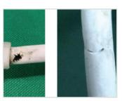
Do not install fixtures with damaged lead wires or accessories. Water ingression can result.
