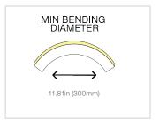
Do not over bend & avoid bending at the first unit of light and connector. Damage to components can result.
