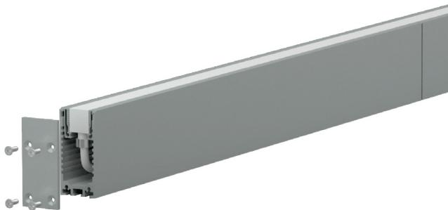
Expanded serrated aluminum profile made from high-quality 6063 thin-wall aluminum, featuring a lightweight structure with concealed cable routing. Raceway space is up to 570mm<sup>2</sup>, providing sufficient room to conceal injection-moulded bottom-feed connectors as well as standard male/female connectors. Suitable for facades where tidiness is required and for installations with limited wiring space.
