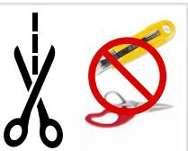
Cut the Vivid Linear Flex Light only at the identification mark using special cutting tools.
