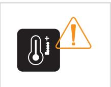
Avoid installing in small, confined spaces warmer than -40°F ~131°F (-40°C ~ 55°C)
