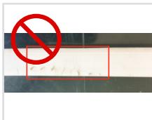
Do not use the product if silicone casing material is damaged.
