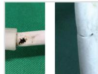
Do not install fixtures with damaged lead wires or accessories. Water ingress can result.
