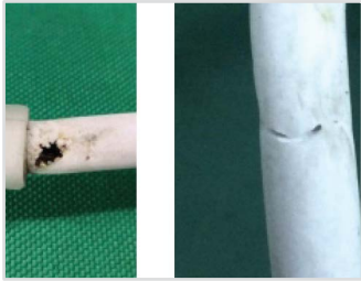
Do not install fixtures with damaged lead wires or accessories. Water ingress can result.
