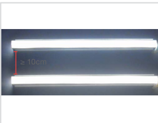
When installing lights in parallel, keep at least 10 cm between them. If they are too close, overheating may occur and could damage the housing material and electronic components.
