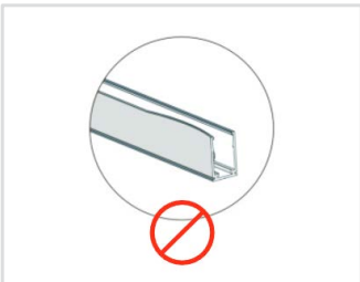
Do not install bent mounting profile.
