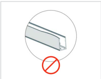
Do not install bent mounting profile.
