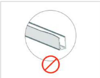
Do not install bent mounting profile.
