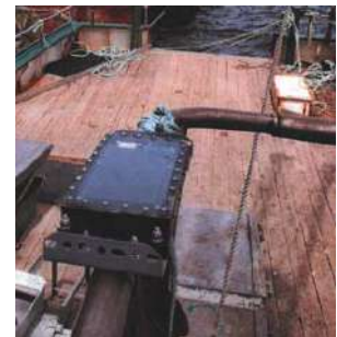
Image Above: Solar-powered deck unit that receives the data from the Moana Sensor
