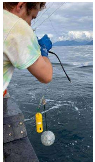
Image Below: Sensor being deployed on a Salmon Trolling vessel line in Southeast Alaska
