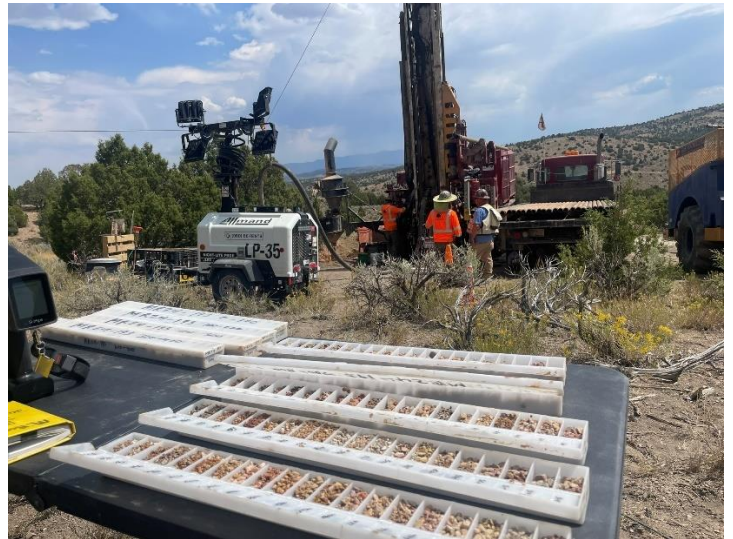
Figure 44: RC chips at the drill site
