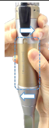
Spot size adjuster (Turn it to adjust the size)
