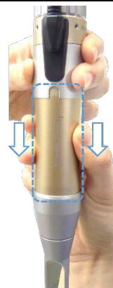
Spot size adjuster (Pull it for size adjustment)
