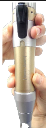
Position of spot size adjuster
