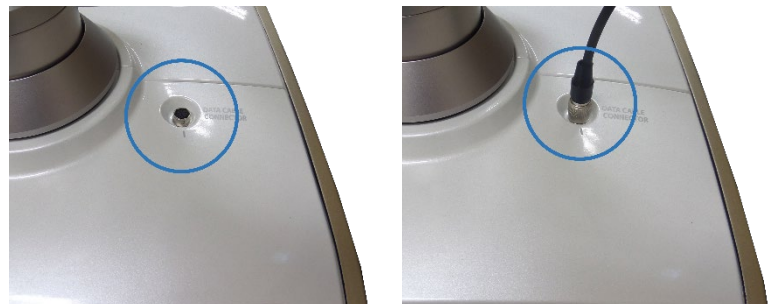
Handpiece cable socket on main unit
