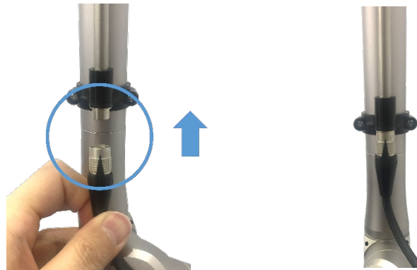
Connection of handpiece cable
