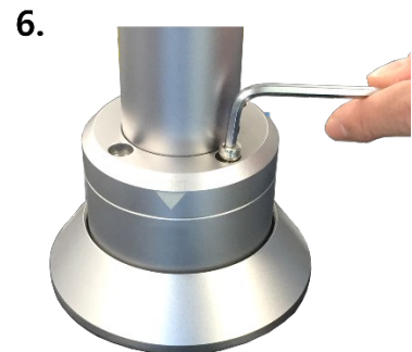
Assembling of articulated arm
