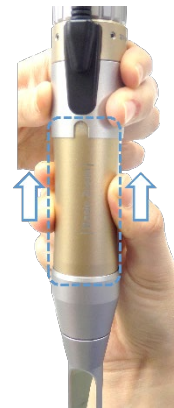
Fixed the spot size adjuster
