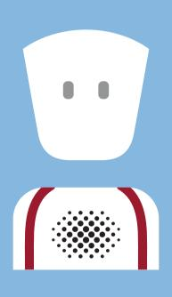
A flashing red light means the AV1 is experiencing connectivity issues. When the lights remains solid white the AV1 has reconnected to the network.
