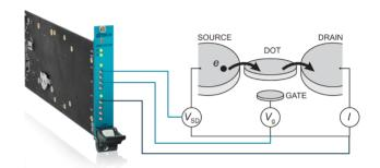
The schematic shows how QSM is used in a typical quantum dot architecture.
