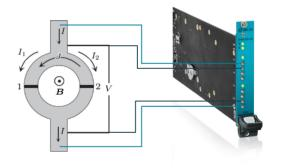
DC-SQUIDs and Josephson junctions are fundamental elements of superconducting qubits. As both devices may operate both at current and voltage biased modes, QSM is an ideal module for such applications.
