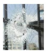
Safety and Security film is engineered for strength. Once installed, it makes the glass less vulnerable by adding a tough layer that will hold the glass together better upon breakage.
