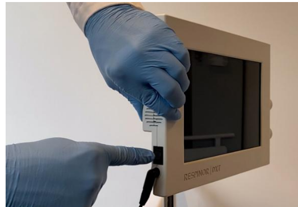
Step 2: Power on the Control Unit by pressing the black power switch.
