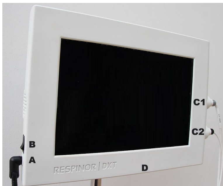
Figure 3. DXT Control Unit. A: Power switch, B: Power supply connector, C1: DXT Anterior Sensor connector, C2: DXT Posterior Sensor connector, D: Service port.
