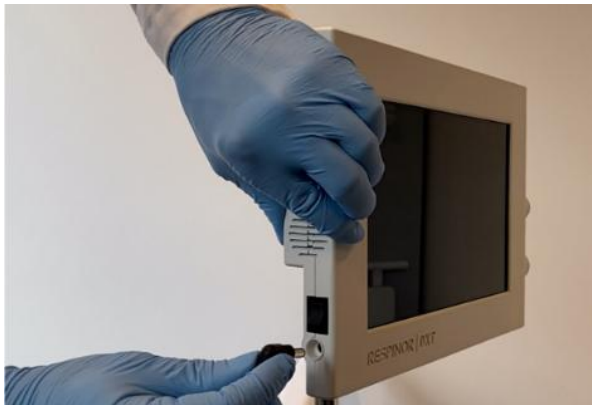
Step 1: Connect the Power Supply on the left side of the Control Unit and connect the power plug to an electrical outlet.
