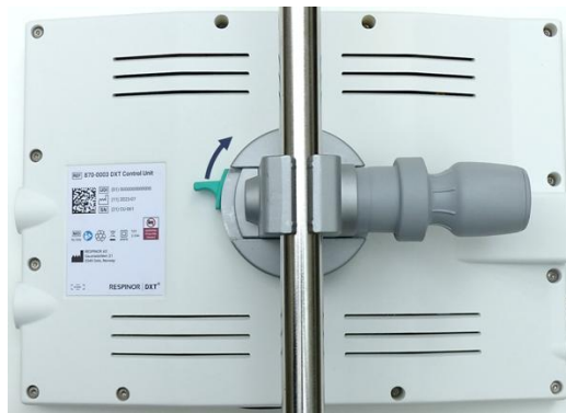
Figure 8. Lift the green handle to release DXT from the Clamp.
