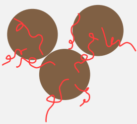
Once particles are saturated, additional polymer is partially bound, leaving polymer loops to effectively bridge particles
