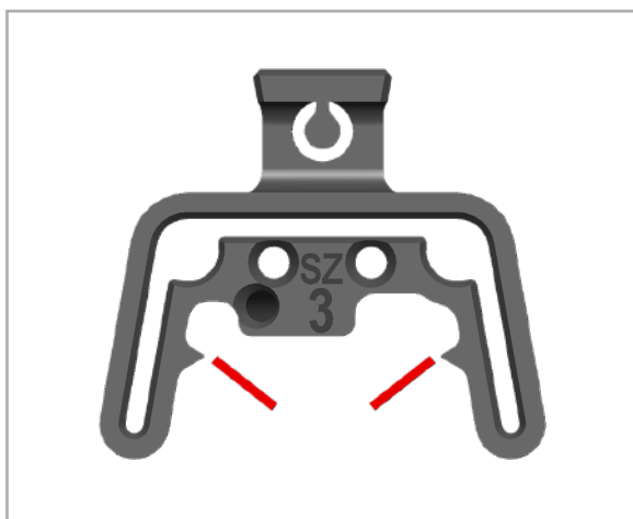
Figure 8 Joint line reference cues
