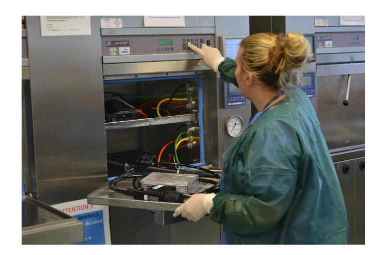
This bank of 6 machines sterilise medical utensils by way of special cleaning process delivered at very high temperature and are critical for patient care services.
