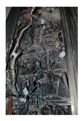
This is one of the machines following a serious internal fire which resulted in significant water and smoke damage as well as the loss of the machine and critical patient care services
