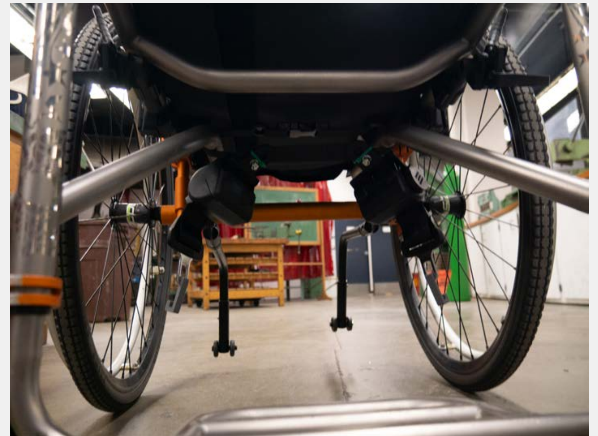
REPURPOSED SEATBELT MECHANISM PROVIDES RETRACTION
