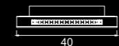
CERCHIO FLUSH ROUND MX15030005-1A NON-DIMMABLE LED 28.8W 1380LM 3000K Φ 40 H 9cm
