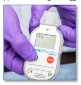
12.11. Place the activated temperature monitor inside the payload compartment under the product bag.
