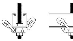
This method is only suitable for use with a 4 way transverse/longitudinal brace. Seismic hooks must be sequenced as shown to align at 45° angle
