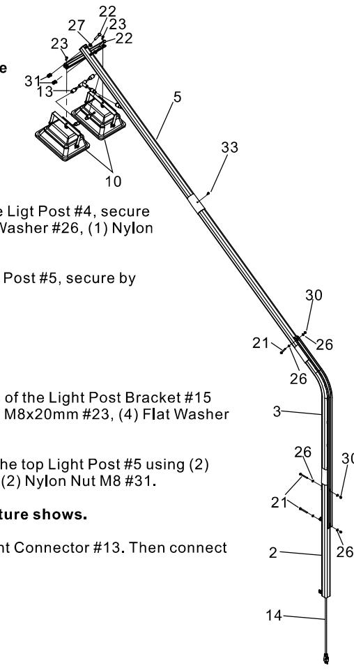
Second, insert the curved light post #3 into the Light Post #4, secure by using (1) Hex Bolt M6x65mm #21, (2) Flat Washer #26, (1) Nylon Nut M6 #30.
