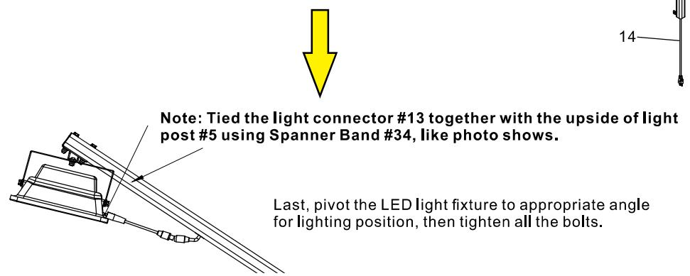
**Note:** Tied the light connector #13 together with the upside of light post #5 using Spanner Band #34, like photo shows.
