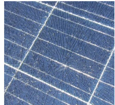
Figure 3. Close-up photo of impact point that broke the glass front of this PV panel
