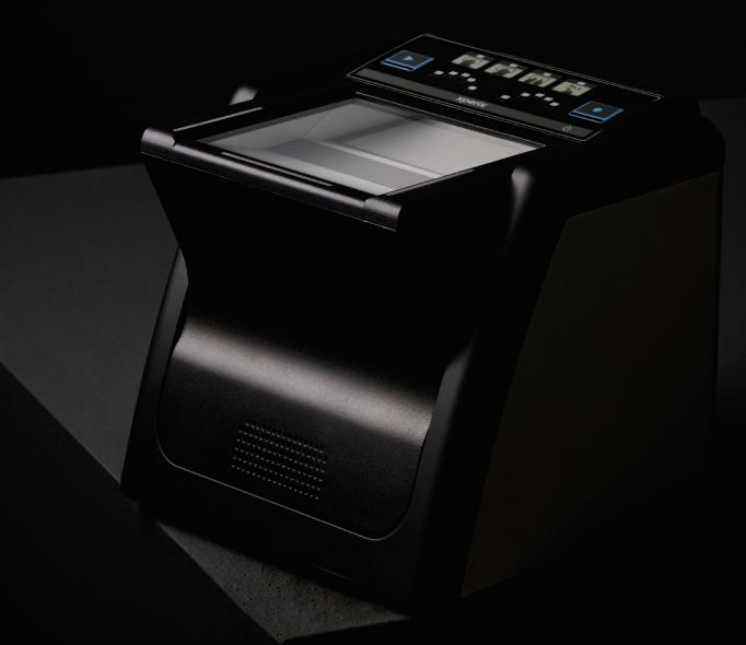
RealScan-G10 is a compact live-scanner for single and ten-print capture. Xperix's advanced optical technology allows high-speed image capturing and seamless image processing. IP54-rated dust and water resistant housing makes it suitable for indoor and mobile environments. With its proven reliability of FBI certification, RealScan-G10 is the perfect portable live-scanner for civil and criminal applications.
