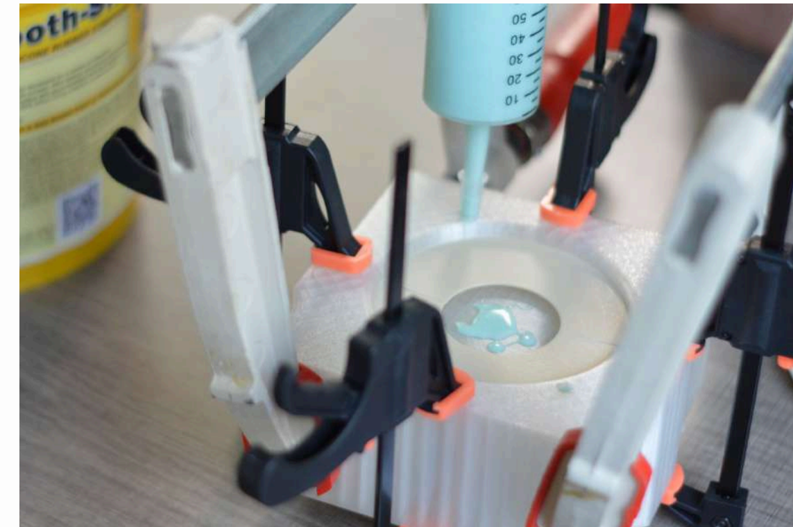
2. Injecting the mold with silicone mix
