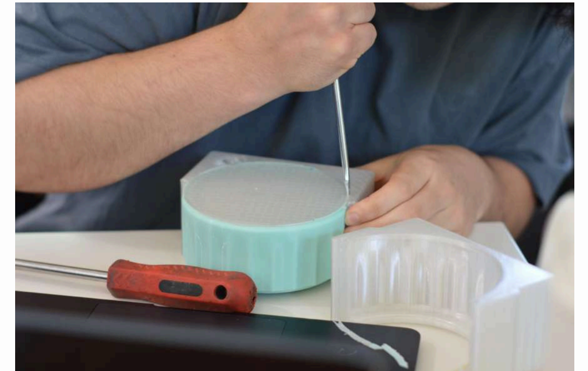
3. Demolding after the silicone has set
