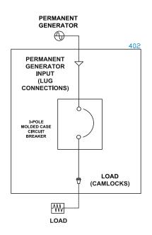
**PERMANENT GENERATOR**  $\bigoplus$ 402-1 PERMANENT **GENERATOR** INPUT (LUG CONNECTIONS) 3-POLE MOLDED CASE CIRCUIT BREAKER LOAD LOAD (LUG (CAMLOCKS) CONNECTION) BEHIND COVER PLATE ₩ LOAD
