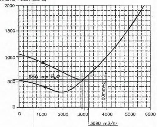
FLOW CAPACITY CURVE, SCMH(Standard cubic meter per hour)
