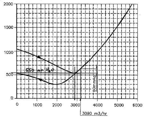
FLOW CAPACITY CURVE, SCMH(Standard cubic meter per hour) (1SCMH = 6.269BBL/hr)
