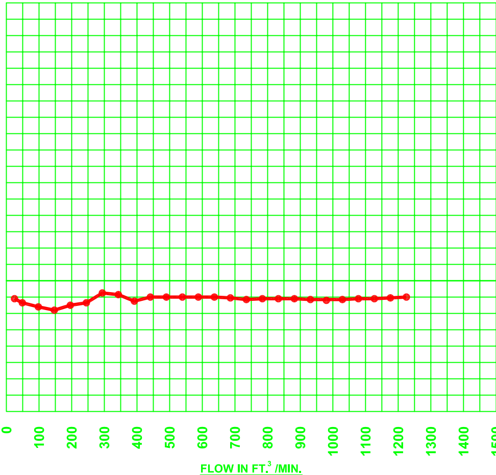
CURVE FOR VACUUM SIDE OF 6" PV VALVE - 0.5 PSI DATA BASED ON AIR FLOW
