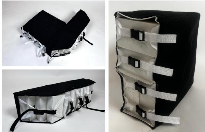
(Top image): This full-scale module demonstrates our final storage unit design. It includes 3D-printed CTBs, adjustable buckle straps, and a Velcro-backed fabric shell. The unit attaches directly to the tensioned circular frame using pre-defined mounting points, confirming proper fit, secure attachment, and spatial efficiency within the inflatable habitat.
