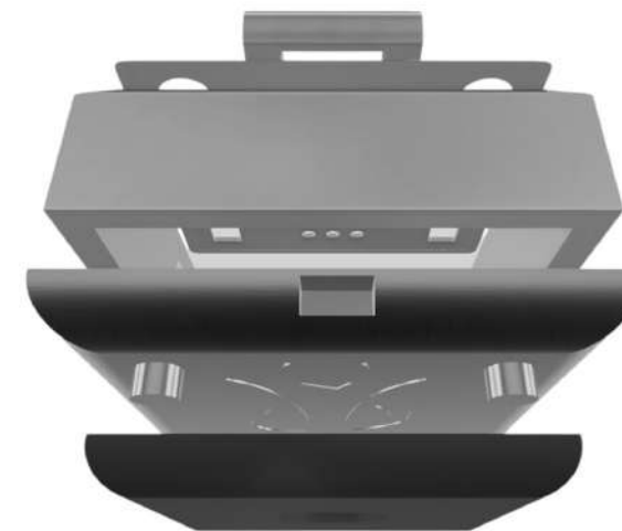
Snap-fit exploded view for clamping
