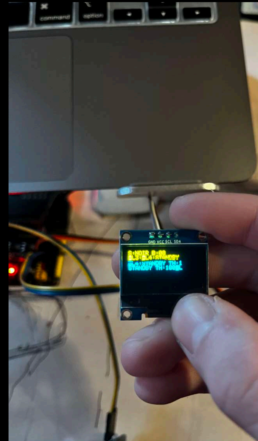
Adding an OLED screen as the LCD screen was too limited in terms of things to display.
