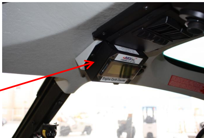
Figure 3 - Installed view of the (optional) cycle counting remote display
