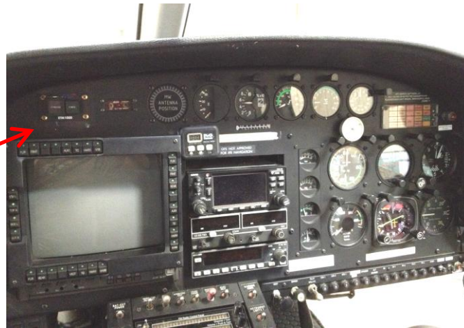
Figure 2 - Installed view of the ETM1000 pushbutton / annunciator
