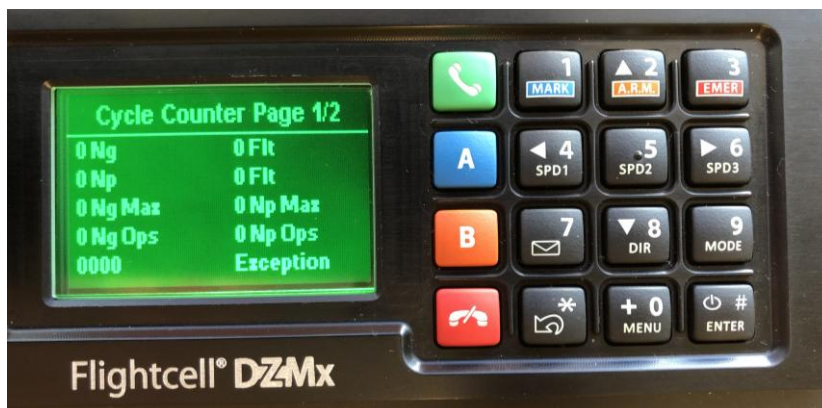
Figure 4 –(Optional) Flightcell DZMx with cycle counting display
