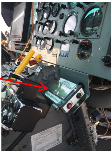
Figure 3 - Installed view of the (optional) cycle counting remote display
