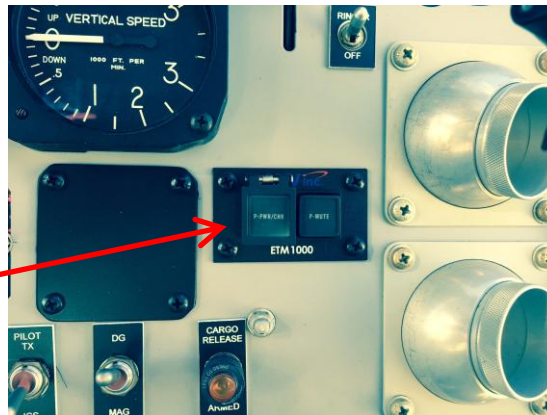
Figure 2 - Installed view of the ETM1000 pushbutton / annunciator
