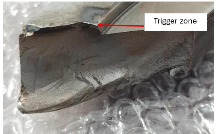
FIGURE 7: MAC A BROKEN RING FRACTURE.
