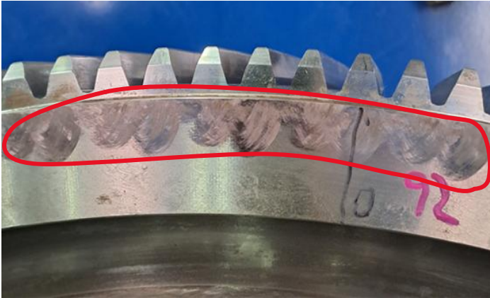
FIGURE 5: 2 SETS OF 92 IMPRINTS ON MAC B BULL GEAR.
