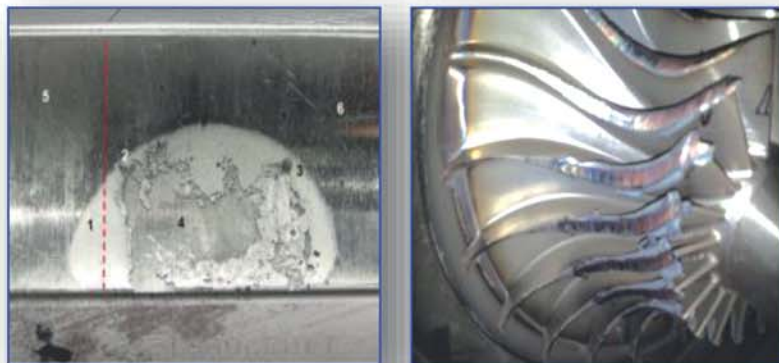
Damaged bearing pad and impeller
