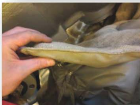
Bottom half cylinder insulation blanket thickness
