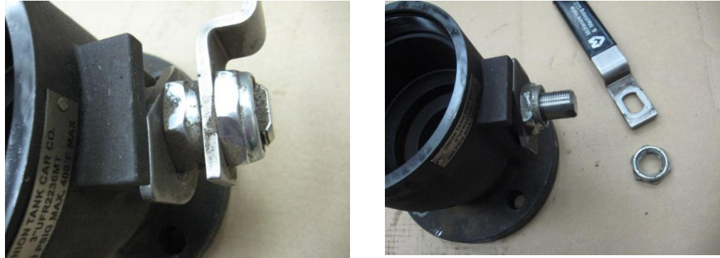
Image 6 – Stem Nut and Handle Removal
