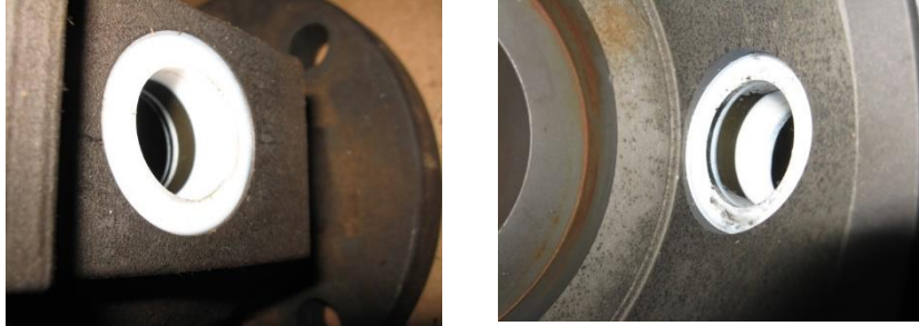
Image 9 – Packing and Thrust Washer Removal
