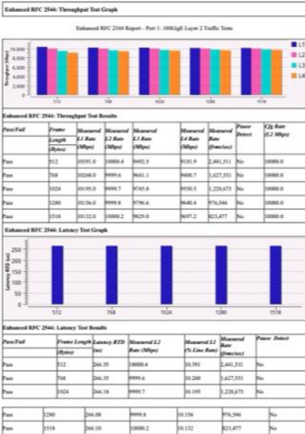
Figure 3 - RFC2544 Throughput and Latency Test Results
