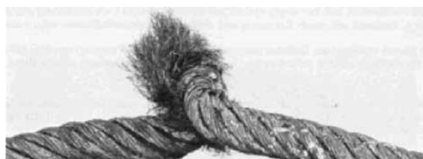
Figure 5: Wire rope with kink
