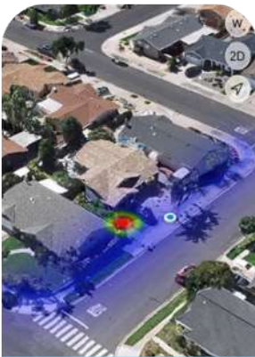
Breadcrumb field-of-view showing areas of zero or elevated methane concentration.
