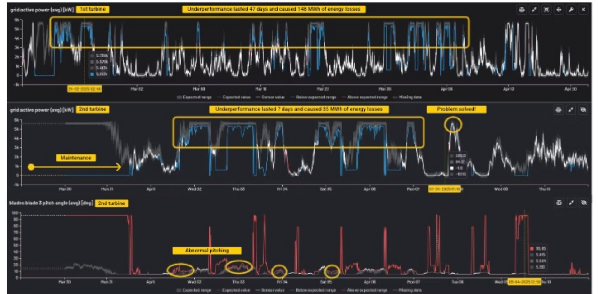
Figure 2 - Normality charts for the grid active powers and the average blades pitch, showing clear deviation from the expected and healthy behaviors
