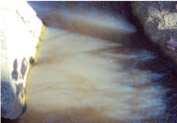
The outfall channel had filled while effluent was discharging. The water quality of the final effluent was turbid and odorous.
