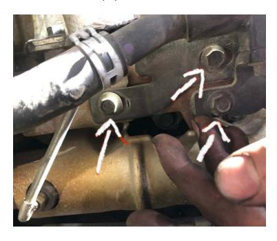
**Step 24:** Pull off the Bypass Valve Assembly including the front section of the cooler plumbing.
