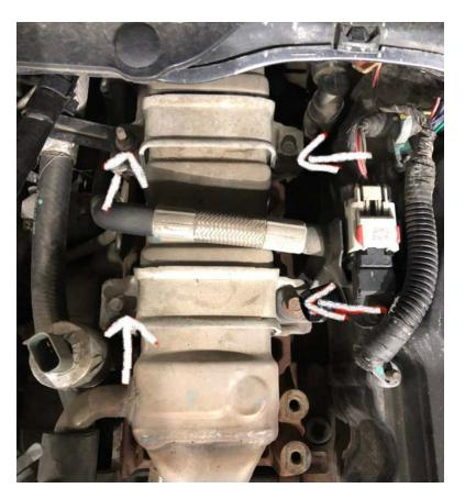
Step 27: On the back left side, use a pry bar to get the transmission dipstick tube hold-down off (68RFE Automatics Only)
