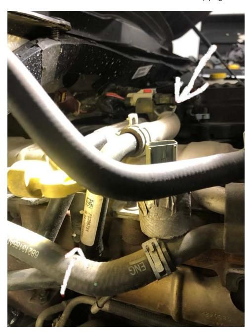
**Step 15:** Remove the intake tube and smaller crankcase tube from the air filter to the turbocharger.
