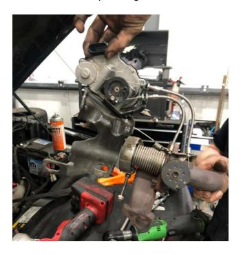
Step 25: Now you can get the 15mm nuts that you had saved to put on the supplied small steel plate and Torque to 37ft-lb.
