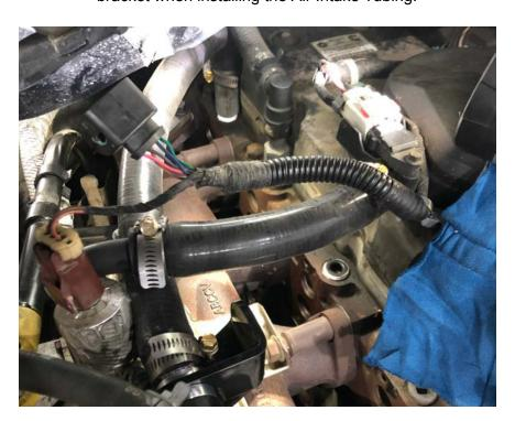
**Step 51:** Make sure you unplug the throttle valve on the rear of the Intake Horn by the DIRTY plate.
