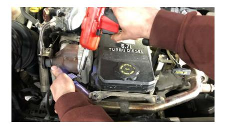
Proceed to break the clamp free with a flat head screwdriver and put back out of the way.
