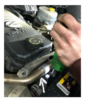
**Step 6:** Now, on the far left side of the EGR crossover tube undo the v-band clamp using an 11mm Deep Socket.
