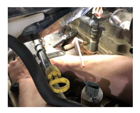
**Step 41:** Grab the supplied aluminum hose adapter, lube it up and press it into the coolant line as seen in the image on the following page.
