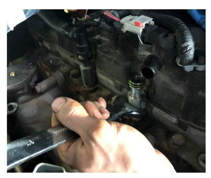
**Step 39:** Grab the Coolant Nipple you removed in the last step and remove the O-Ring and put Teflon Tape on the threads and have it ready to place into the plug you are removing in the next step.
