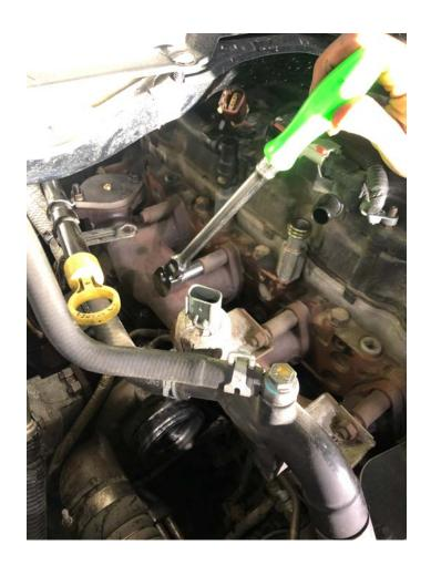
Step 35: Thread in the stud with the Factory Collar and tighten the 15mm supplied nut,
