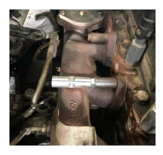
**Step 37:** Get your supplied ½" NPT Plug ready by wrapping it in Teflon Tape to plug the hole you're about to make.
