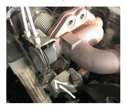
**Step 19:** Remove the remaining heatshield bolts using an 8mm socket.
