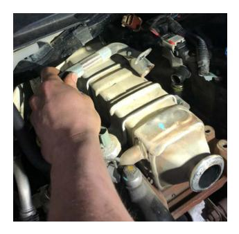
**Step 31:** Use a pry bar to release the cooler from the bracket and pull the cooler up and forward to remove it.
