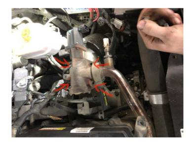
**Step 5:** Next, is (1x) One 8mm bolt directly in-line with the oil cap in between the EGR cross over the tube and the radiator hose. As seen in the photo below, use your ratchet to press down on the rad hose to get in. This one is a bit tough to get at!
