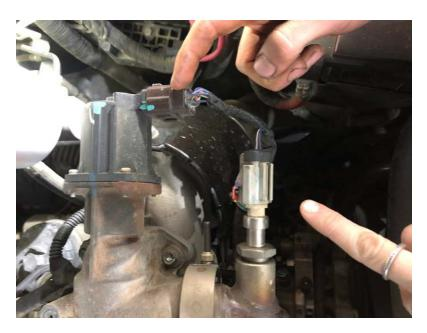
**Step 4:** Once the EGR is disconnected, remove (x4) bolts holding the EGR Valve on top of the intake horn using a 10mm socket.
