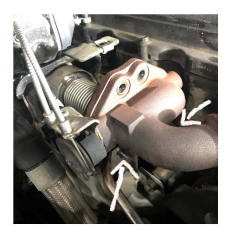
**Step 18:** Now you can pry the heatshield off the one stud and bend it out of way to pull the front piece off.
