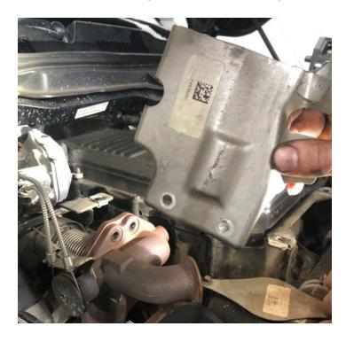
**Step 20:** Spray Penetrating Oil on the two (x2) 15mm nuts holding the Front of the EGR to the exhaust manifold and let them rest (maybe grab yourself a beer while they soak.).
