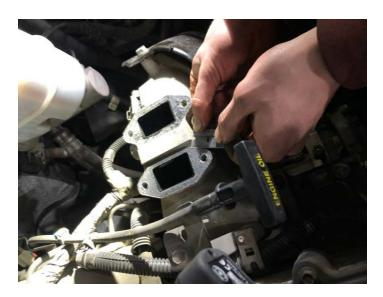
**Step 9:** Once the surface is as clean as possible, place both new gaskets on with the larger Aluminum anodized plate using the socket head bolts provided.
