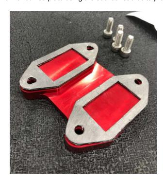
Step10: Place the Logo side of the plate up, with the gasket on your intake horn and use a 6mm Allen Head to Torque to 18ft-lb
