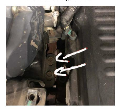
Step 23: Remove the three (x3) bolts on the other side of the EGR Cooler
