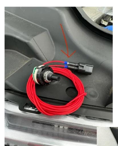
10. Once the switch has been pinned to the supplied connector, disconnect the factory harness from the charge air temp sensor.
