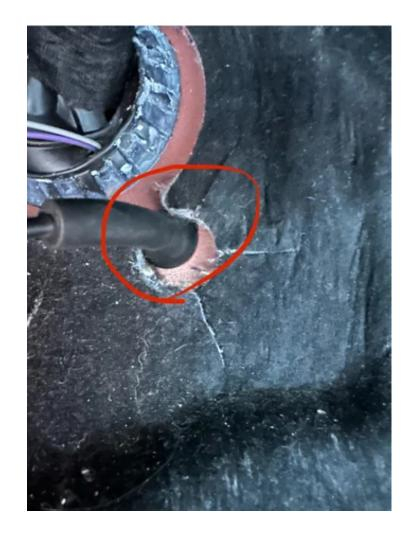
3. Locate the hood release cable where it is fed through the firewall behind the brake pedal.
