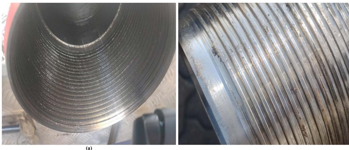
Figure 8—Images from the AR device camera during Tubular Inspection Activity: (a) shows the Box side, and (b) shows the Pin side, where high-resolution photos assist remote experts in identifying any visual damage.
