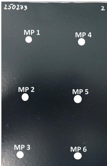
Figure 1: P1.2 – Positions at which DFT-measurements were taken
