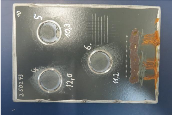
Figure 8: P1.10 – Cross cut + pull-offs
