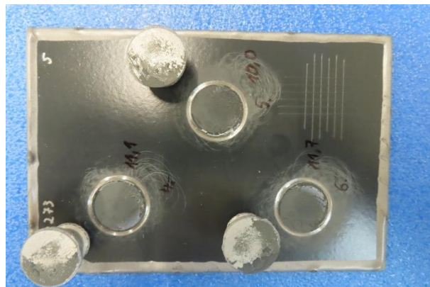
Figure 3: P1.5 – Cross cut + pull-offs
