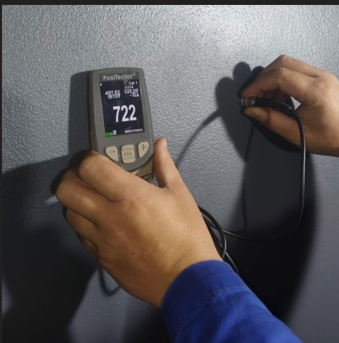
DFT Paint Thickness Measurement
