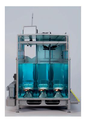
The Turbo Scalder 1070 applies a powerful downwards water flow to ensure fast immersion and effective opening of the entire feather pack to facilitate water penetration.
