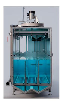
The AirJet Scalder 1050 uses air to agitate the water inside the tub, which effectively reduces the water density and causes the product to immerse while the air bubbles ruffle the feathers and allow the hot water to penetrate.
